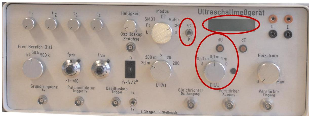
**Fig. 3.2: Ultrasound measurement electronics. The parts used for the temperature measurement are marked in red.**
